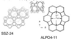
I propose to study the Xe NMR spectra for sealed samples of Xe in crystalline zeolite SSZ-24 which has a one-dimensional channel structure and then to consider other systems with channels having elliptical cross sections such as ALPO4-11. Again, studies at different mole ratios of Xe to zeolite and variable temperature will be done for a comprehensive comparison with simulations.
