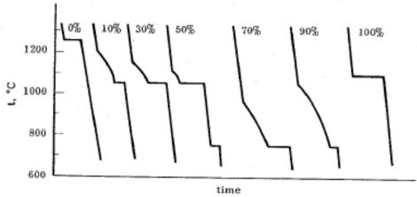
Construct the most reasonable semi-quantitative freezing-point diagram, label all phase regions, and give the probable formulas of any compounds that are formed.
