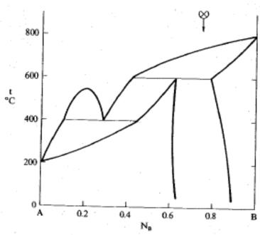
Label all regions as to the phases present, using "A" or "B" to denote pure solid A or B, and  $C_1$ ,  $C_2$ , etc., for pure solid compounds, and use  $\alpha$ ,  $\beta$ , etc. to denote solid solutions rich in A, B, and so on. Use L to denote a liquid solution (or  $L_1$ ,  $L_2$ , etc.). Sketch the cooling curve for a system of the composition indicated by  $\otimes$  in the figure above, and state what phases appear or disappear at each halt or break.
