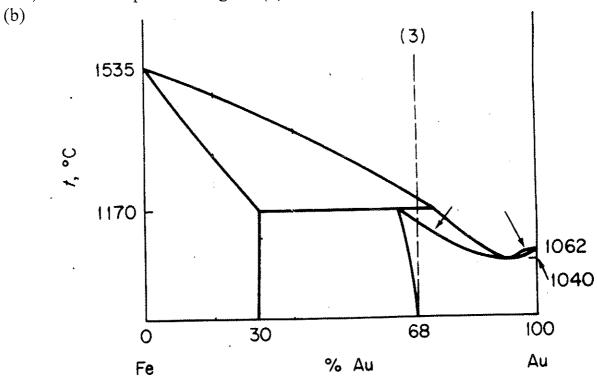
**Draw a <u>labeled</u> cooling curve** for a melt of composition 68% Au, along vertical line (3) as seen above:
