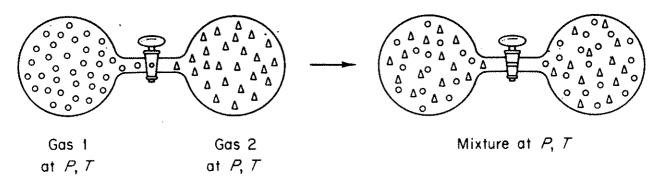
Fundamentals:  $d\mathbf{G} = Vdp - \mathbf{S}dT$ ; when dT = 0,  $d\mathbf{G} = Vdp$ ; for one mole of a pure substance, this becomes  $d\mu = V_m dp$ . Integrating between lower limit of 1 bar and upper limit of p,  $\int d\mu = \int V_m dp = \int (RT/p)dp$  for an ideal gas, leads to  $\mu(g, T, p) = \mu^{\Theta}(g, T, 1 \text{ bar}) + RT \ln(p/1 \text{ bar})$
