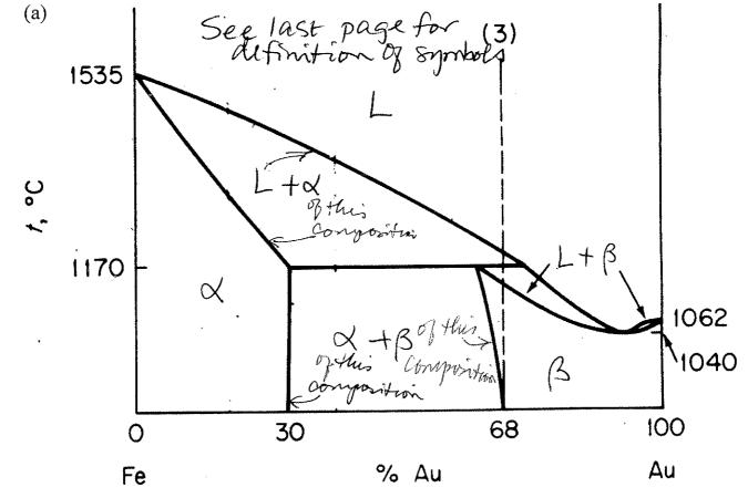
Write the number of degrees of freedom (in addition to pressure) in each region, line, intersection point in diagram (b): Answer use F' = C - P + 1 = 3 - P {except at the 0% and 100% Au vertical lines, at which C=1}
