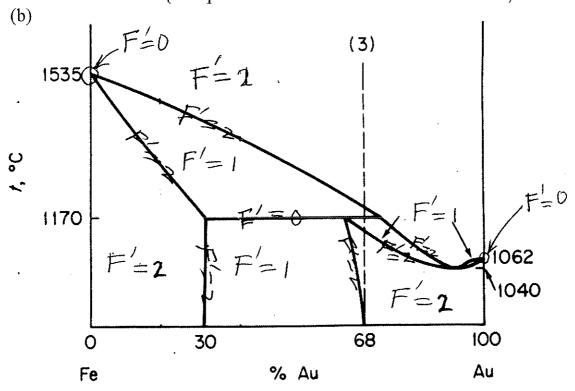
Draw a <u>labeled</u> cooling curve for a melt of composition 68% Au, along vertical
