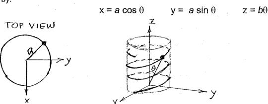
Since there are t turns, at the bottom end of the helix  $\theta = 0^{\circ}$  and at the top end of the helix  $\theta = t(2\pi)$ .
